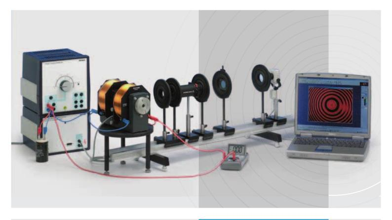
Discover the splitting of the spectral lines of atoms within a magnetic field with the Zeeman effect
