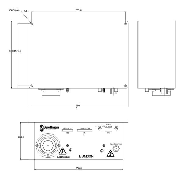
The EBM30N must be fitted in a unit and secured in position using the mounting brackets provided. A safety interlock should be used to prevent access to the unit when it is operating.
