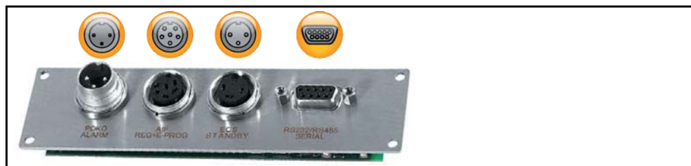
Com.G@te internal interfaces: POKO, AIF, ECS, RS232/RS485 (left to right).
