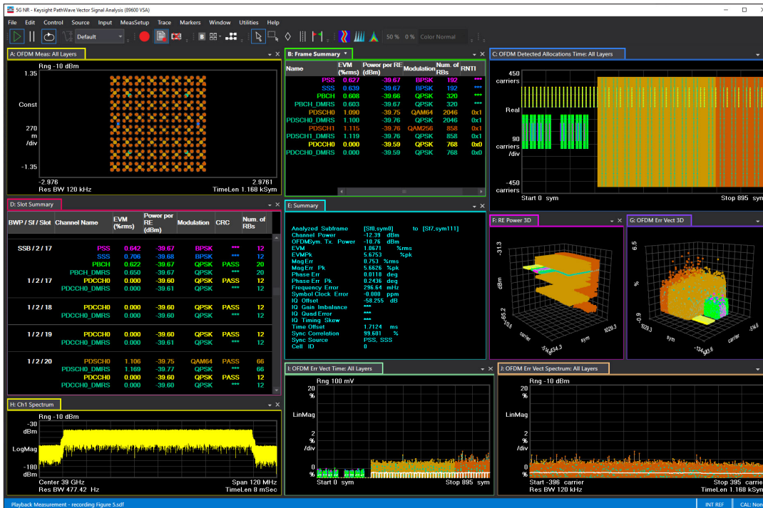
Figure 5. Example analysis of a downlink signal, at 39 GHz center frequency, with SS/PBCH, PDCCH and multiple PDSCHs.
