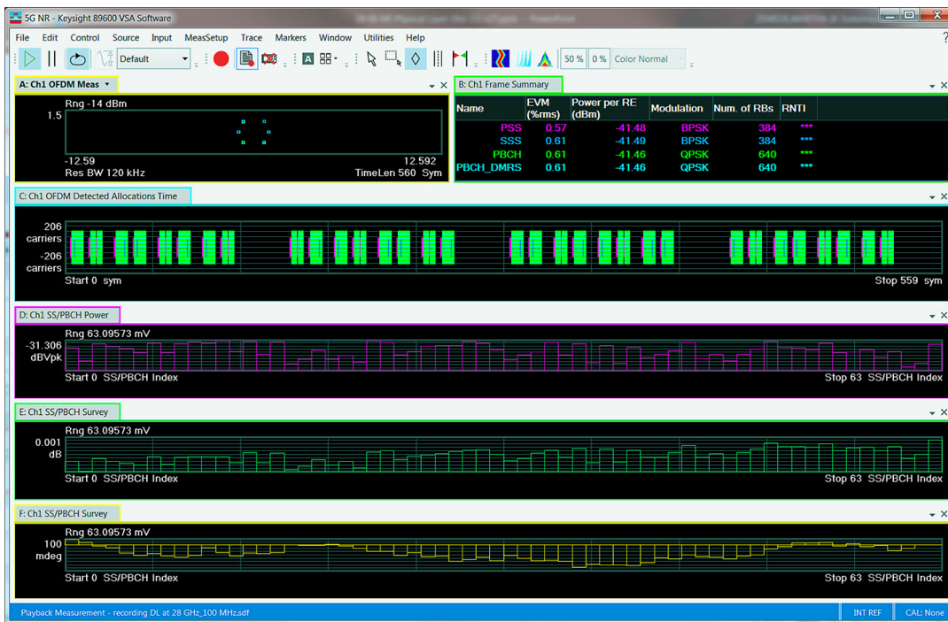
Figure 8. Example of SS/PBCH dedicated measurements to measure power and phase of each SS/PBCH active indices.
