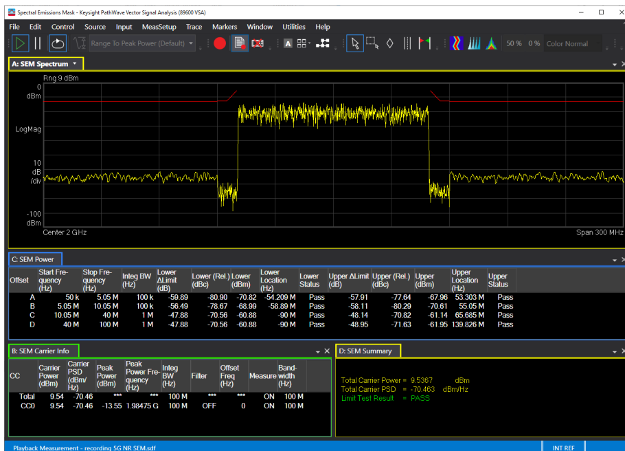
Figure 14: SEM measurement of a single carrier 5G NR signal
