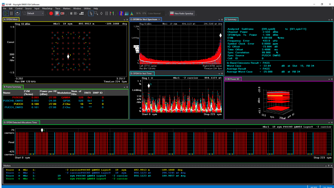
Figure 7. Example of coupled markers across multiple color-coded traces in different measurement domains.
