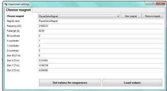
Frequency  $\rightarrow$  Selects the excitation frequency of the HF pulses and the mixing frequency of the system.
