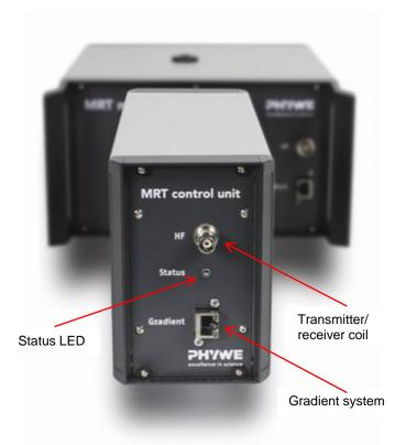
Fig. 2: Front of the control unit
