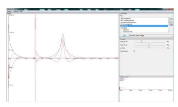
The program has four areas: the area for selecting the lessons, the area for adjusting the parameters in a lesson, the time-resolved representation of the sequence in the lesson, and a graphical representation of the last measurement results
