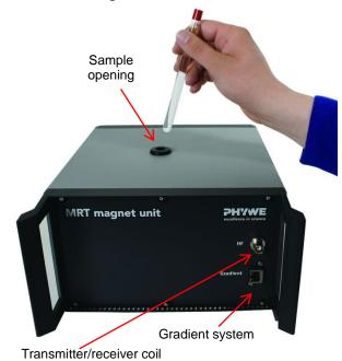
Fig. 4: Front of the magnet
