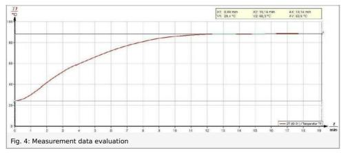
The values in the table or the function "Survey" d can be used in combination with the measurement curve in order to determine the temperature increase.
