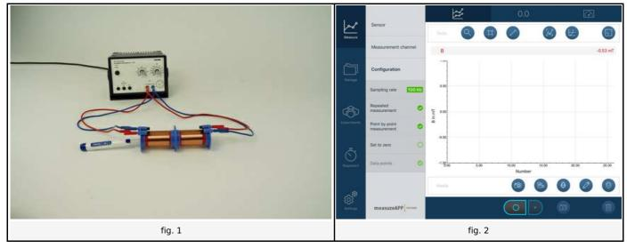
Build the experiment as shown in fig. 1. The coils are connected in parallel. Make sure the polarity is the same for both coils. The coil connections are each outside, so the winding of the two coils are opposite. Make sure, the current of the two coils having the same corkscrew direction. Connect your tablet to the Cobra SMARTsense magnetic field sensor. Select point by point measerement [Configuration-> Point by point measerment (fig. 2)].
