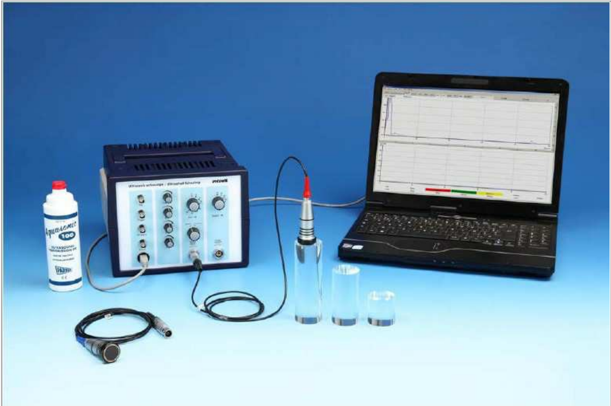
Fig. 1: Equipment for ultrasound velocity measurements, experimental set-up
