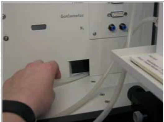
Fig. 3: Tubes laid through the working channel
