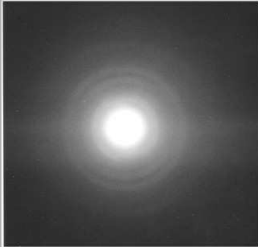
Fig. 7: Debye-Scherrer pattern of a zirconium foil. Thickness of the sample: 0.05 mm. Exposure time: 2.5 h. Mo X-ray tube: UA = 35 kV; IA = 1 mA
