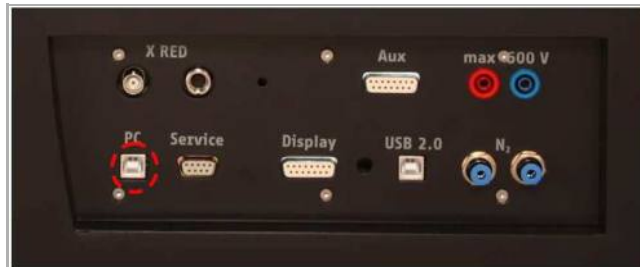
Fig. 4: Connection of the computer
