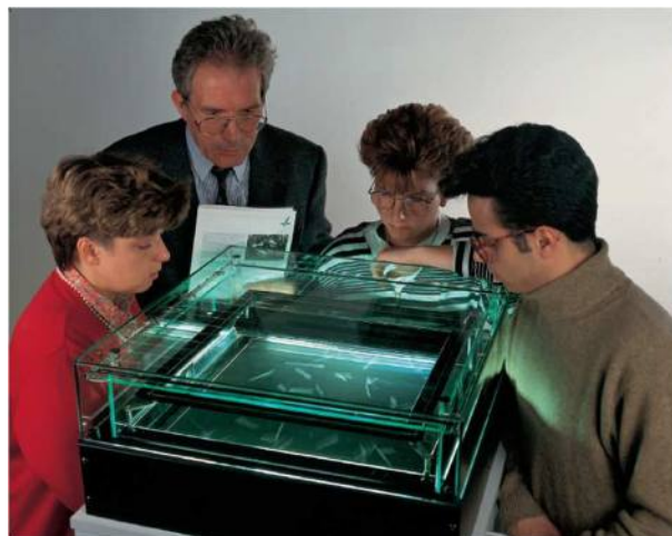
Fig. 1: Experimental set-up: Diffusion cloud chamber.
