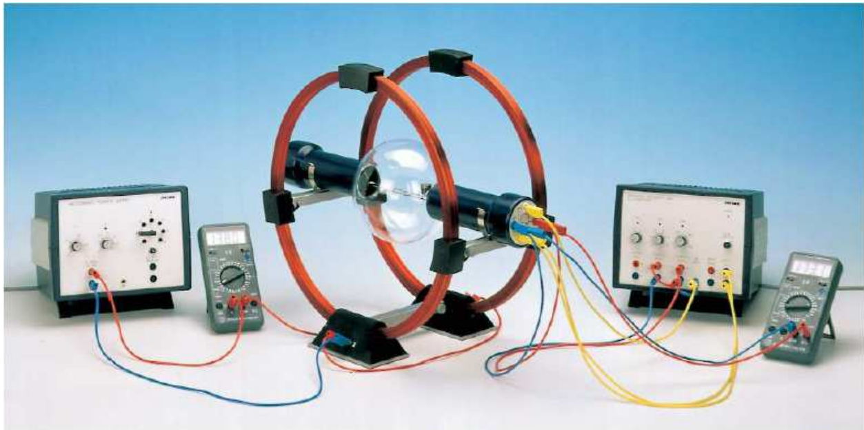
Fig.1: Experimental set-up for determining the specific charge of the electron.
