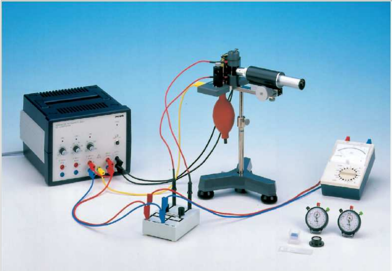
Fig. 1: Experimental set up for determining the elementary charge with the Millikan apparatus.
