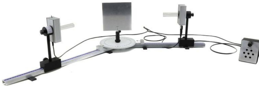
Fig. 9: Experiment set-up (law of reflection).
