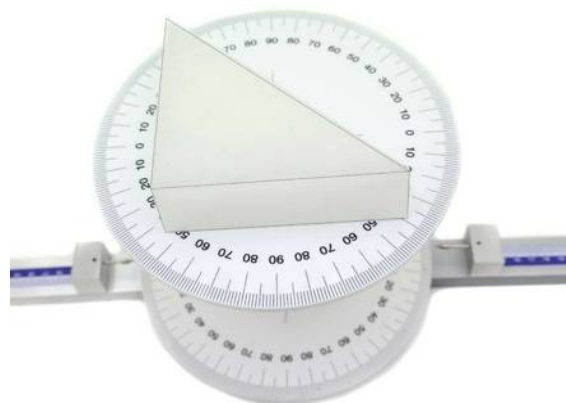
Fig. 6: Positioning of the prism on protractor with pin.
