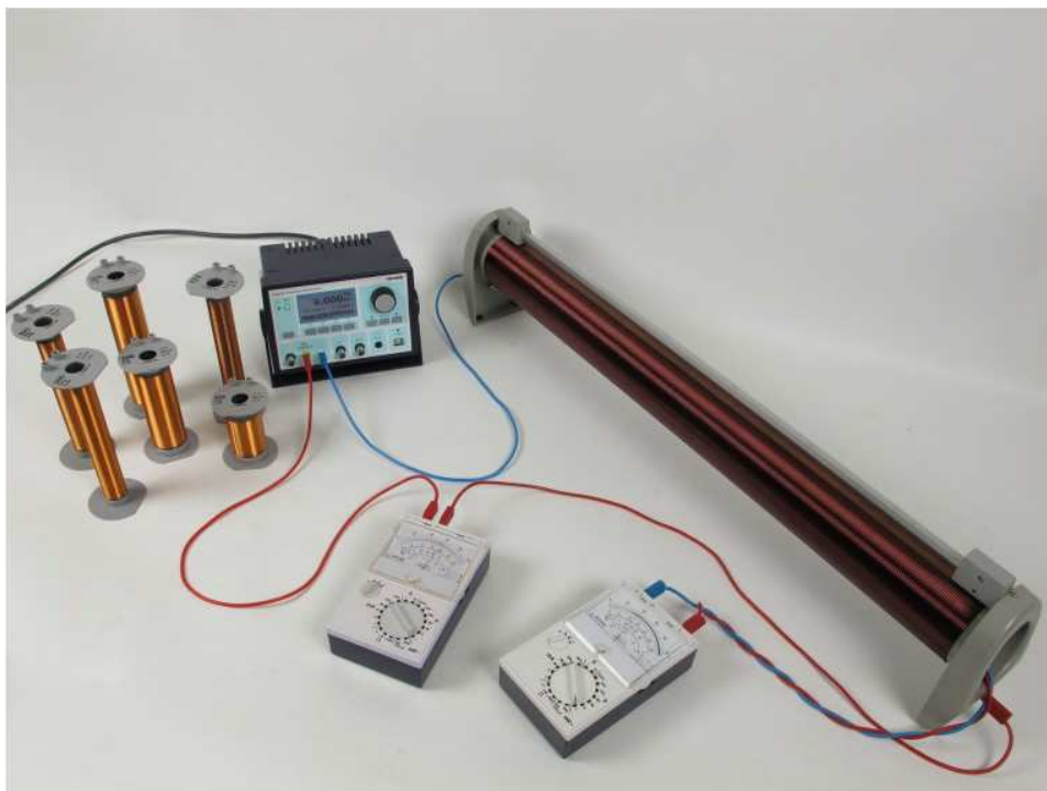
Fig. 1: Experimental set-up with one induction coil slid into the field coil.
