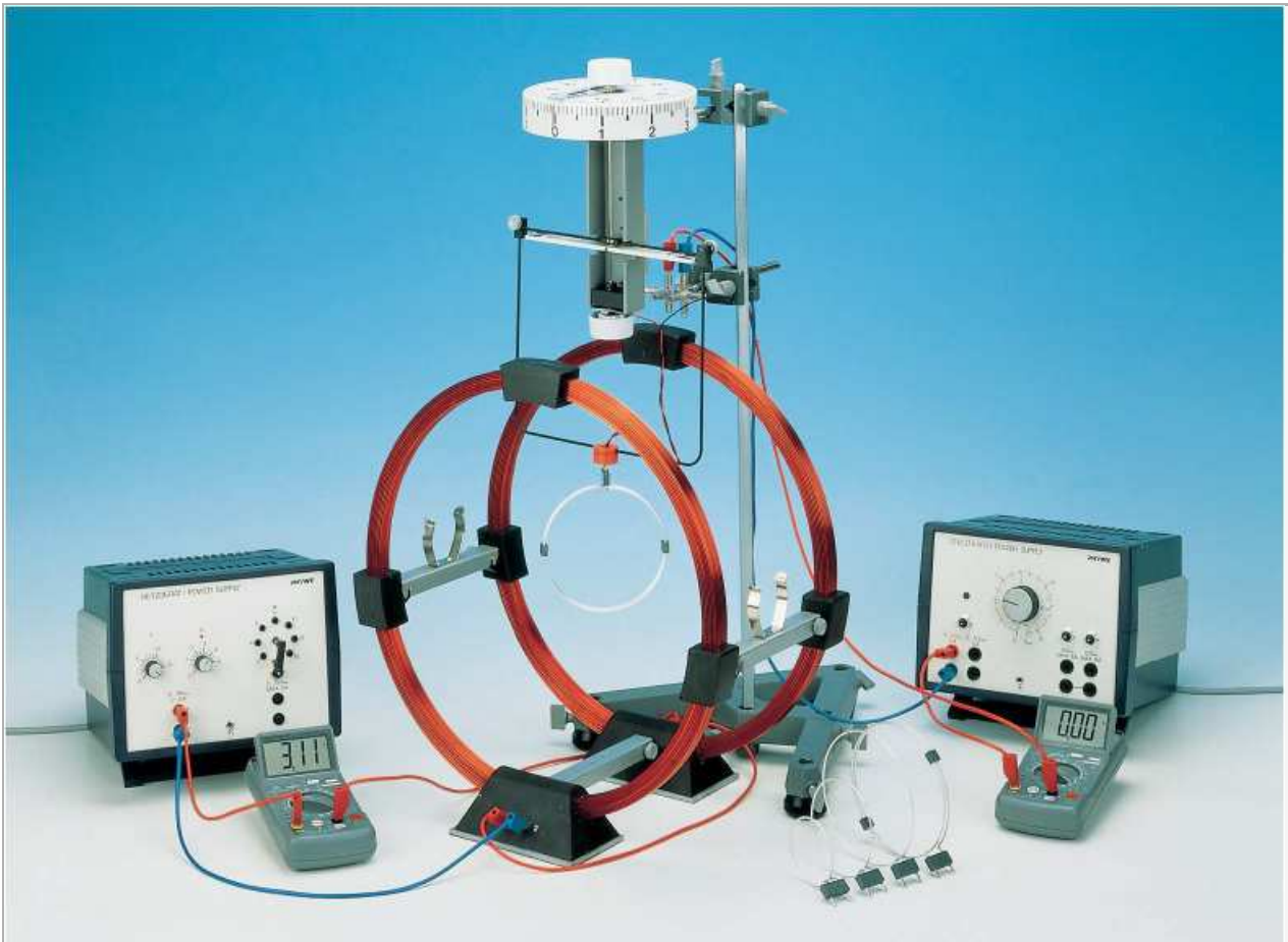
Fig. 1: Experimental set-up for determining the torque due to a magnetic moment in the magnetic field.
