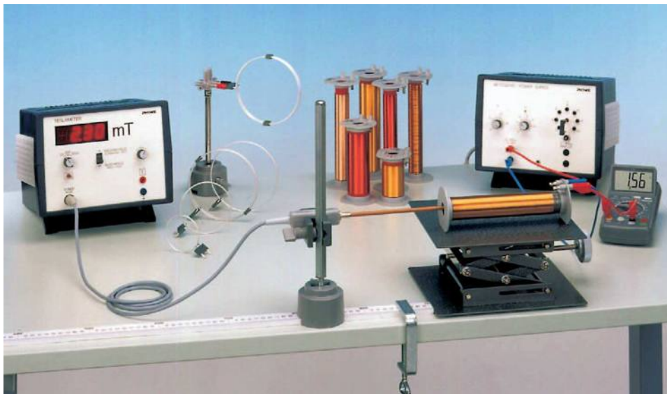
Fig 1: Experimental set-up for measuring a magnetic field.
