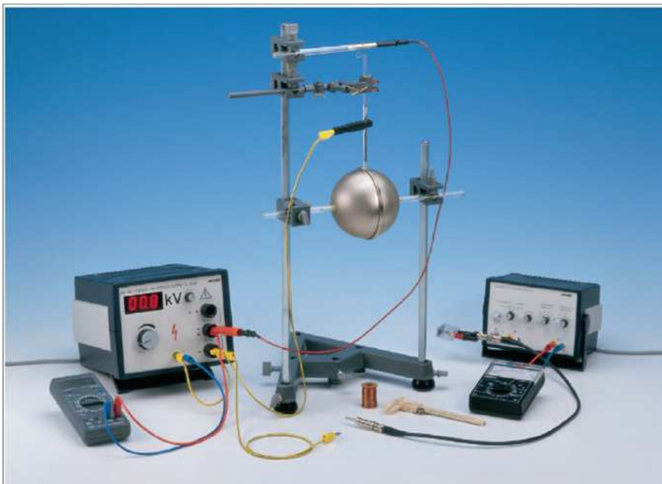
Fig. 2 : Part of the experimental set-up used to determine the capacitance of a spherical capacitor.
