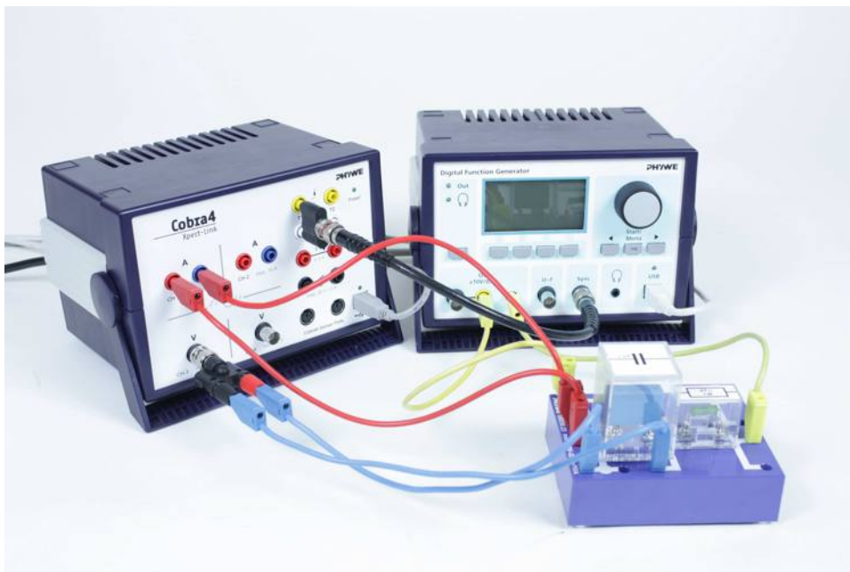
Fig. 1: Experimental set-up for measuring the current when a capacitor is being charged.
