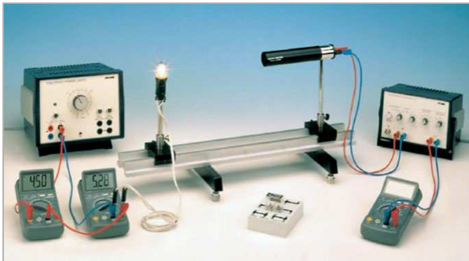
Figure 1: Set-up for experimental verification of Stefan-Boltzmann's law of radiation.
