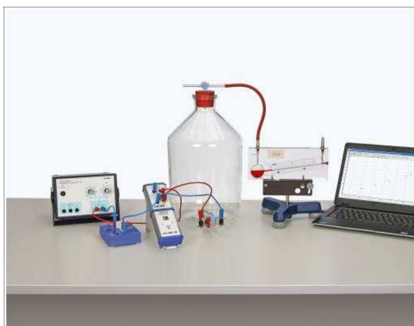
Fig. 1: Experimental set-up for the determination of C_V .
