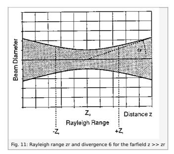
The reason for this is that the ratio of the beam diameter with regard to z has not been normalised. Let's consider, for example, a He-Ne laser (632 nm) with a beam radius of  $w_0=1mm$  at the exit of the laser. For the Rayleigh range  $2\,z_r$  we get:
