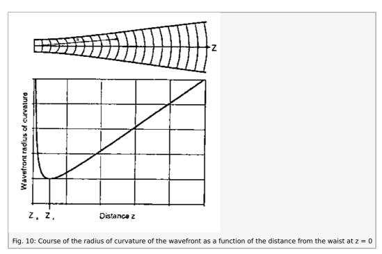
This context is reflected by Fig. 10. At  $z=z_r$  the radius of curvature has a minimum. Then R increases with 1/z if z tends to z=0. For z=0 the radius of curvature is infinite. Here the wavefront is plane. Above the Rayleigh length  $z_r$  the radius of curvature increases linearly. This is a very essential statement. Due to this statement a parallel beam only exists at one point of the light wave, to be precise only in its focus. Within the range
