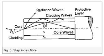
Fig. 5 reveals some basic facts which can be seen without having solved Maxwell's equations. Starting from geometrical considerations we can state that there must be a limiting angle  $\Theta_c$  for total reflection at the boundary between cladding and core.
