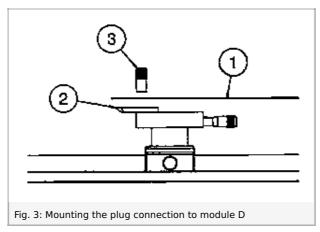
After eliminating the insulation from both fibre ends by scratching, the cut and cleaved fibre (1) is to put into the groove of holder (2) and carefully fixed with the magnet (3).
