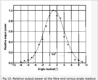
Tig 13. Relative output power at the hore end versus angle readout.
