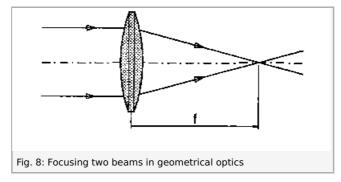
Real parallel light beams do not exist in reality and plane wave fronts exist only at a particular point. The reason for the failure of geometrical optics is the fact that it has been defined at a time where the wave character of light was still as unknown as the possibility to describe its behaviour by Maxwell's equations. To describe the propagation of light we use the wave equation
