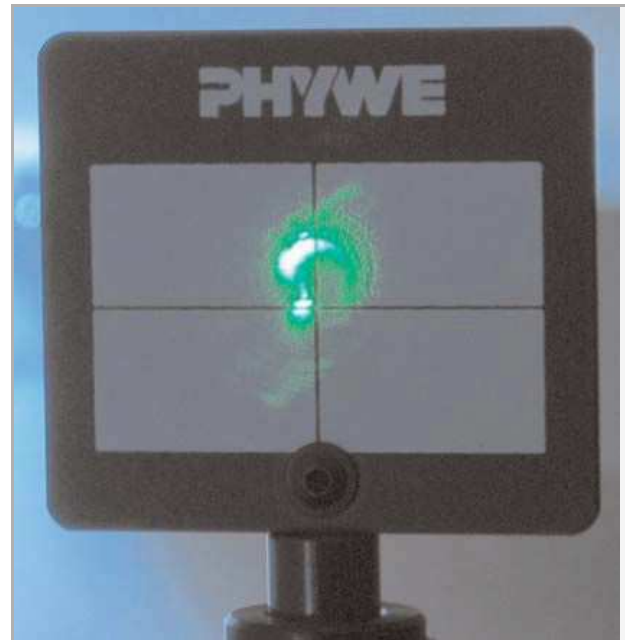
Fig. 7: Bad laser tube alignment
