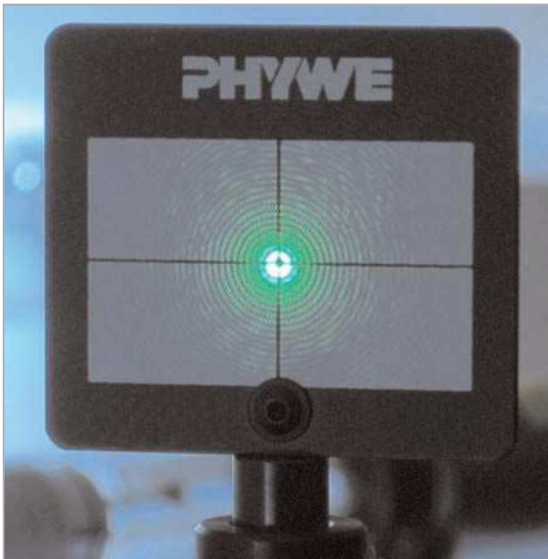
Fig. 6: Good alignment of the adjustment beam
