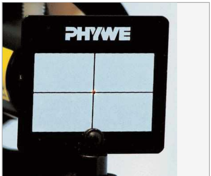
Fig. 10: After beam walking the beam passes almost completely the hole in the left diaphragm
