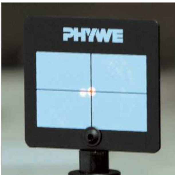
Fig. 9: Beam centered on the right diaphragm with ghost beam visible left of it
