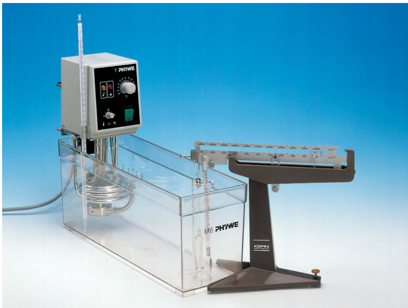
Fig. 1: Experimental set-up for determining density with the Mohr balance.
