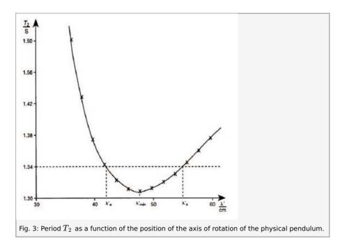
In Fig. 3, the modification of the moment of inertia and the shifting of the center of gravity due to the displacement of the bearing sleeves over the support rod was not taken into account (however, the basic pattern remains unchanged). This error becomes evident during the control measurement of period  $T_1$  around axis of rotation 1, the value of which,  $T_1(\lambda_a)$ , is obviously different from the value obtained for the symmetrical case  $T_1(\lambda_s)$ .
