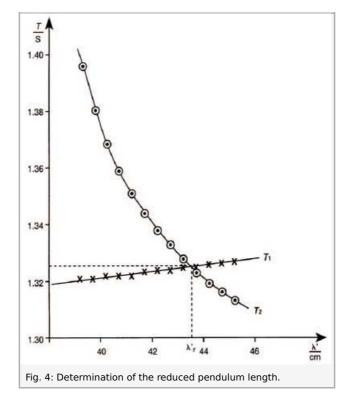
Thus, terrestrial gravitational acceleration g can be determined from the coordinates of the point of intersection in Fig. 4. The values  $T = T_1 = T_2 = (1.325 \pm 0.001) \, \mathrm{s}$  and  $\lambda_{\mathrm{r}} = (43.6 \pm 0.1) \, \mathrm{cm}$
