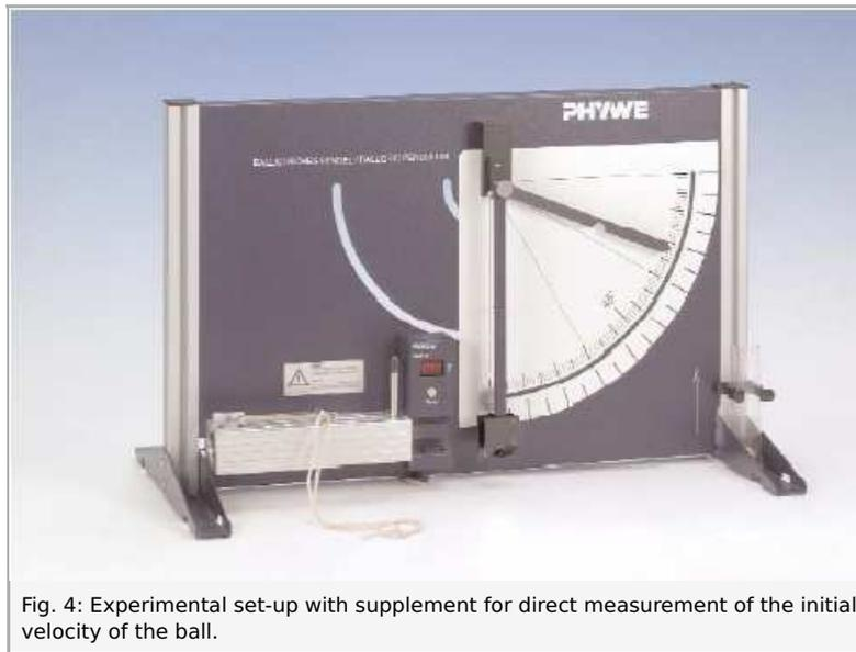
Fig. 4: Experimental set-up with supplement for direct measurement of the initial velocity of the ball.
