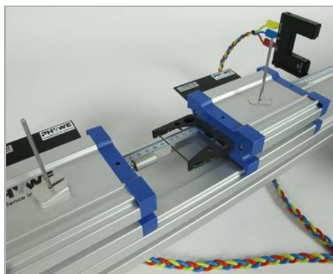
Figure 6: Completed collision prior to reaching the second light barrier
