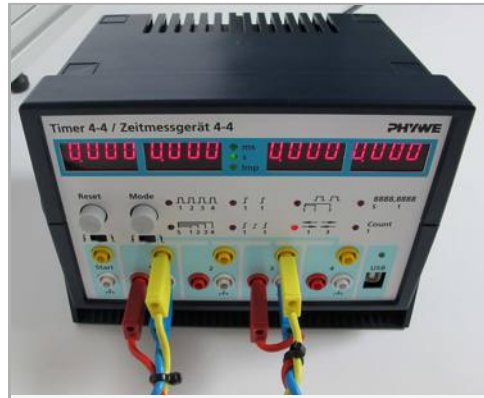
Fig. 4: Connection of the light barriers
