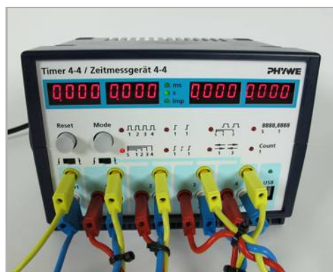
Fig. 7: Connection of the light barriers and starter system
