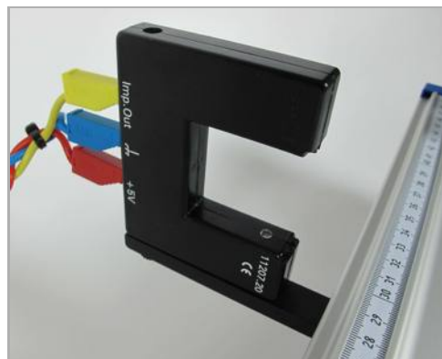
Fig. 3: Installation of the light barriers on the demonstration track
