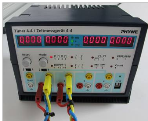
Fig. 4: Connection of the light barriers
