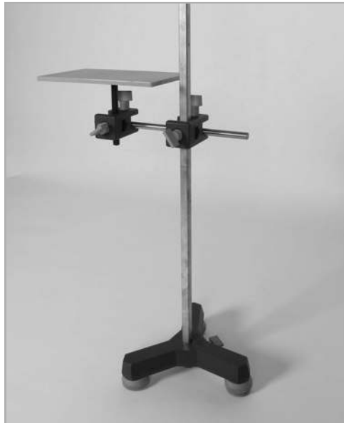
Figure 8: Plate for stopping the weight holder at variable heights
