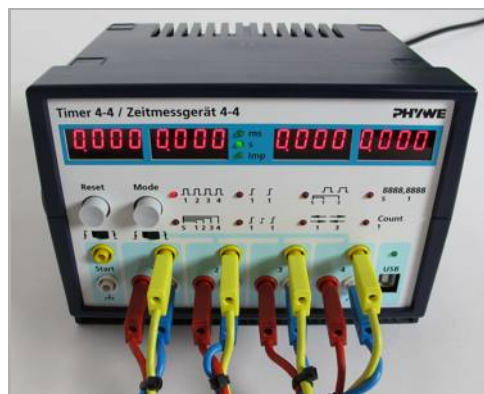
Fig. 7: Connection of the light barriers
