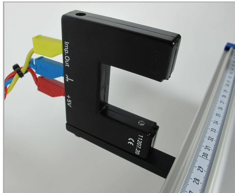
Fig. 5: Installation of the light barriers on the track
