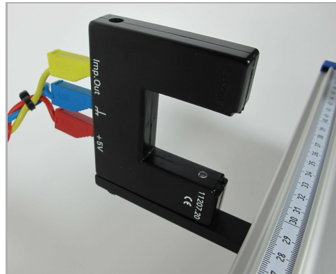
Fig. 5: Installation of the light barriers on the demonstration track
