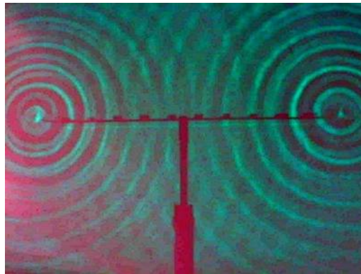
Figure 3: Snapshot as shown in Fig. 1. The interference pattern of the two circular waves can be clearly recognised. As this is a photo the resulting image is like that seen in stroboscopic lighting. The shortening of the wavelength in the area of the standing wave can therefore not be identified on the photo.
