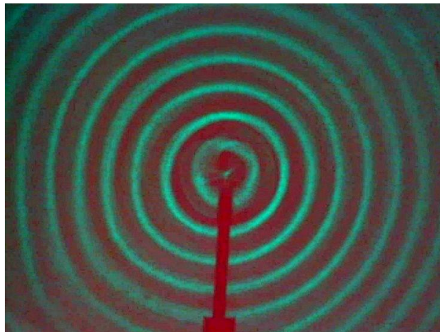
Figure 5: Snapshot according to the arrangement from Fig. 1. The circular waves produced by the single wave generator can be clearly recognised.
