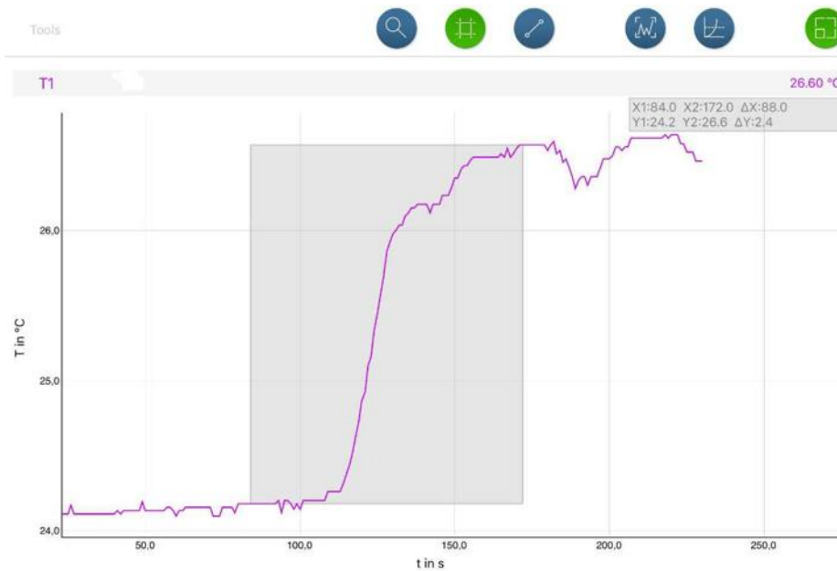
Fig. 2: Behaviour of the temperature display over time, with the measureApp "Survey" tool switched on. Example for brass.
