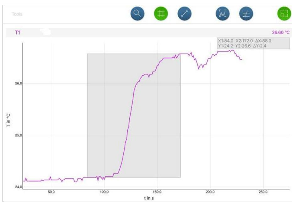
Fig. 2: Behaviour of the temperate display over time, with the measureApp "Survey" tool switched on. Example for brass.
