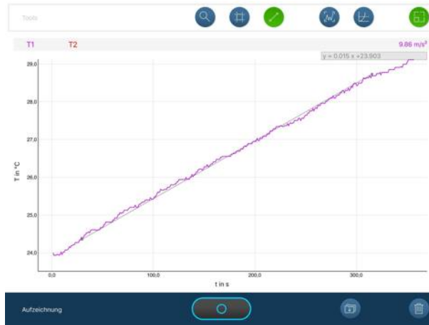
Fig. 3: Behaviour of temperature against time with electric heating, analysed with the "Regression" tool in the measureApp.
