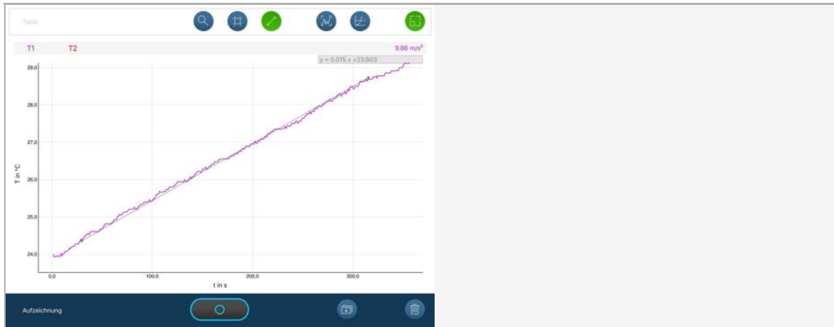
Fig. 4: Behaviour of temperature against time with electric heating, analysed with the "Regression" tool in the measureApp.
