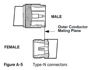
Therefore the mechanical specifications of Type-N connectors give a maximum protrusion of the female contact fingers in front of the outer conductor mating plane and a minimum recession of the shoulder of the male contact pin behind the outer conductor mating plane.
