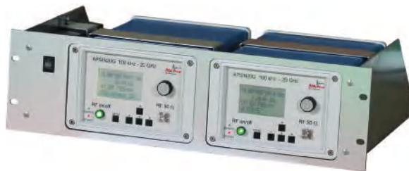
3HU 19" RACK-MOUNT KIT: mounting 2 portable units
