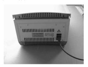
8. Switch on the device at the power supply switch. The lid opens automatically.
