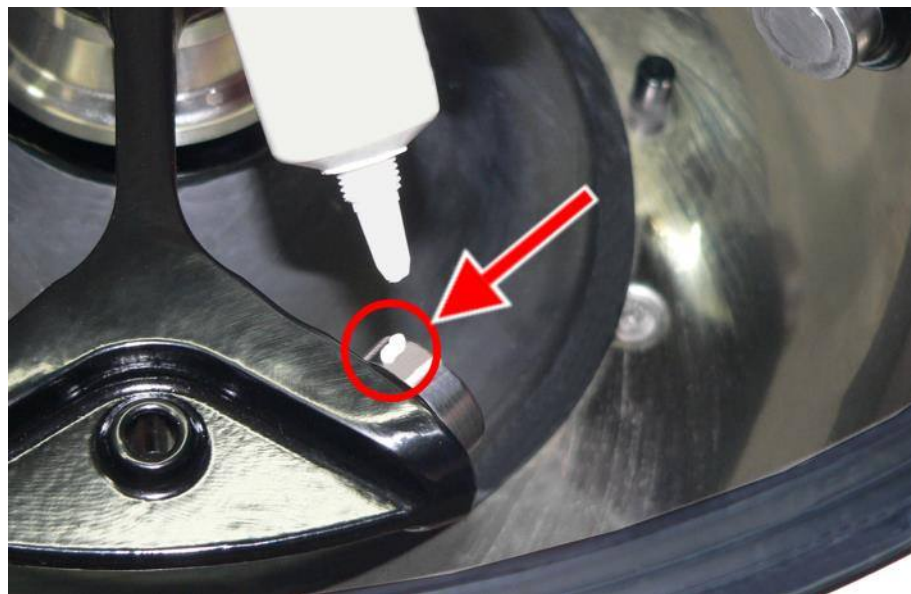
Fig. 30: Sufficient quantity of grease for one bolt
