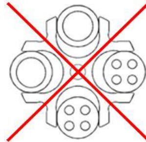
Fig. 6: Permissible and impermissible loading of a swing-out rotor with vessels of various sizes (example illustration)
