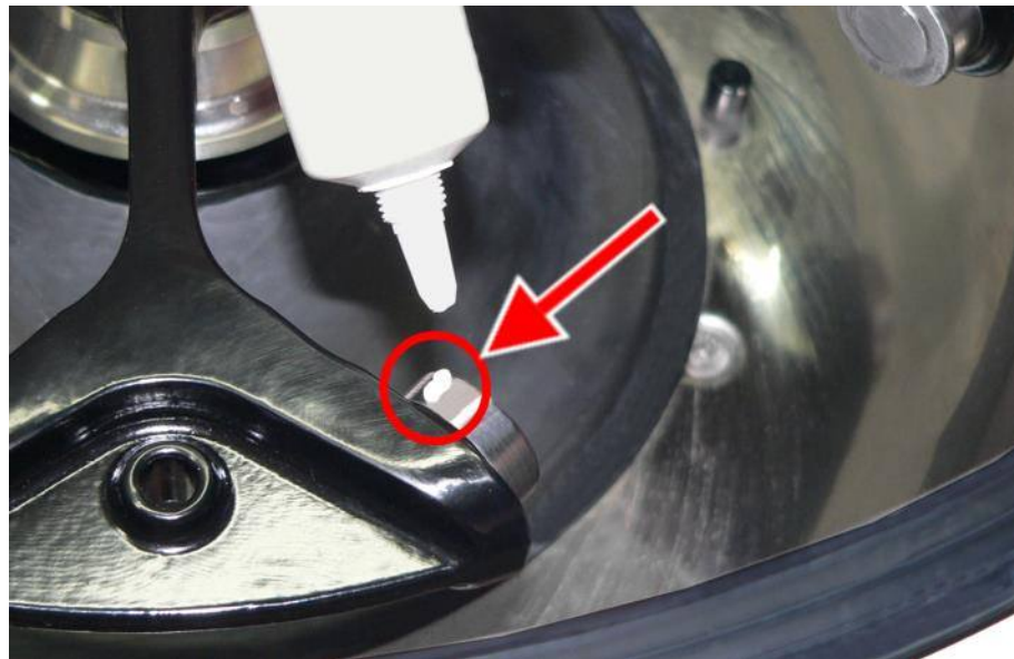
Fig. 30: Sufficient quantity of grease for one bolt
