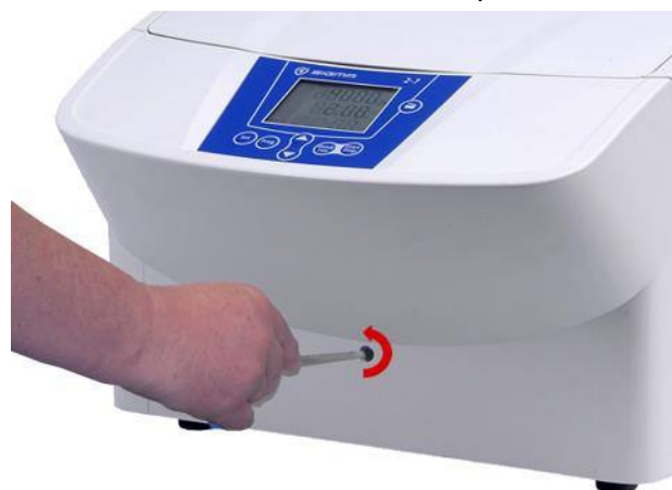
Fig. 11: Manual release of the lid lock
