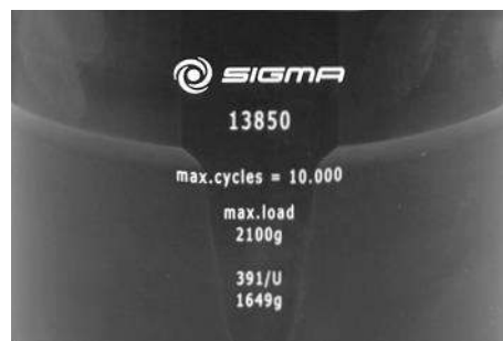
Fig. 4: Different service life – engraving on the bucket/rotor
