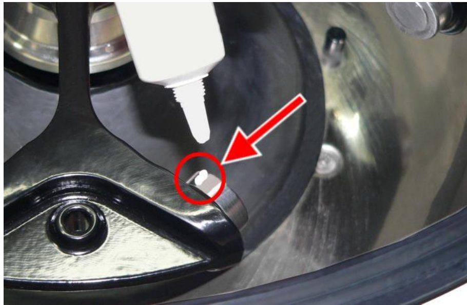
Fig. 29: Sufficient quantity of grease for one bolt
