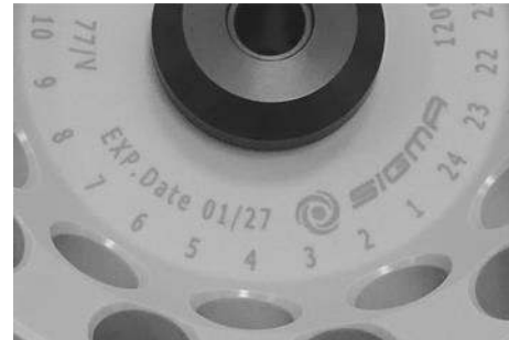
Fig. 4: Different service life – engraving on the bucket/rotor
