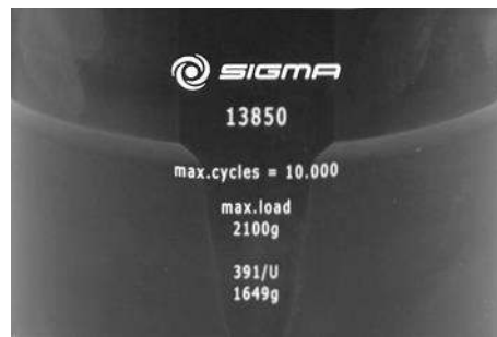
Fig. 4: Different service life – engraving on the bucket/rotor
