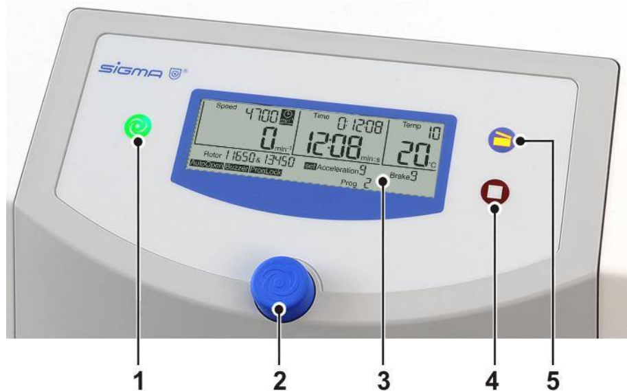
Fig. 9: User interface of the Spincontrol L control system
