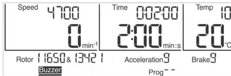
Fig. 21: The sound signal "Buzzer" is activated
