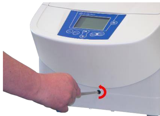
Fig. 9: Manual release of the lid lock
