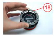
Remove the lock ring (18), incl. screws, from the measuring/transmission unit and remove all soiling.
