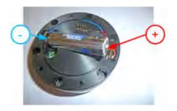
Remove the old battery and insert the new battery (2). Battery type: 1.5 V / AA
