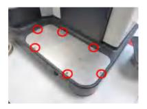
**1.** Remove the layer of rubber on the work surface and loosen the 6 screws with which the plate is attached to the housing.
