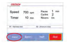
When the mill is switched on, the values of the last milling are displayed. You can make various settings as described below by clicking on the [Menu] button.
