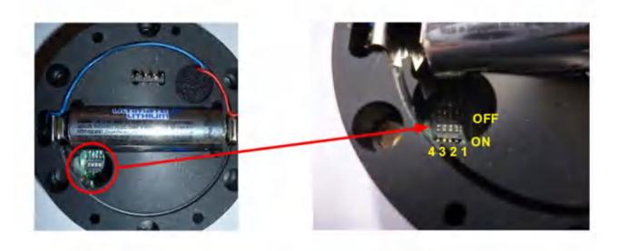
The switches illustrated are all in the **OFF** position (actuator cams set to OFF).
