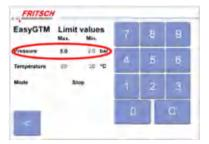
Click on the Max. and Min. fields in the 'Pressure' section and enter the maximum and minimum pressure. If the minimum pressure (14 bar) is reached, the devices goes into cooling mode or stops until the pressure falls below the minimum pressure limit. Once the minimum pressure limit has been reached, grinding continues as normal.
