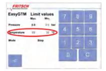
Click on the Max. and Min. fields in the 'Temperature' section and enter the maximum and minimum temperature. If the maximum temperature is reached (125° C), the device goes into cooling mode or stops until the temperature falls below the minimum temperature limit. Once the minimum temperature limit has been reached, grinding continues as normal.
