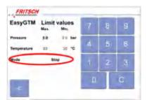
You can use the 'Mode' menu item to select how the PULVERISETTE 5 premium line is to respond to the temperature or pressure limit being reached.
