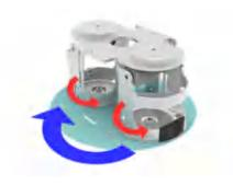
The grinding stock is crushed and ground by grinding balls in a grinding bowl. The centrifugal forces from the rotation of the grinding bowls around their own axis and from the rotating support disc act on the contents of the grinding bowl which consists of grinding stock and grinding balls.
