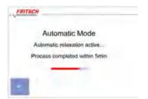
A screen with a progress bar is displayed during automatic unclamping. This indicates approximately how much longer the unclamping process will take.
