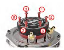
Tighten the hexagon screws crosswise with a torque spanner (1) until it disengages! To be on the safe side, re-tighten all screws again after initially tightening them. All screws are secured against becoming loose during the grinding process once they have been tightened with the torque spanner as described.
