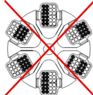
Fig. 23: Permissible and impermissible loading of an angle rotor and a swing-out rotor (example illustration)
