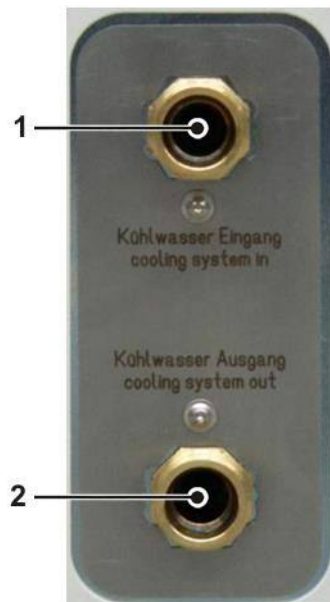
Fig. 18: Connections for the water cooling system
