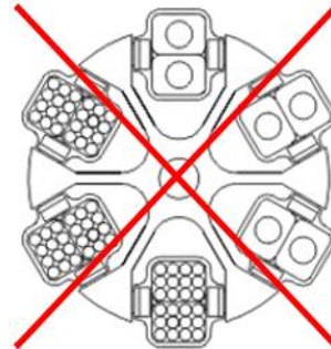
Fig. 22: Permissible and impermissible loading of a swing-out rotor with vessels of various sizes (example illustration)
