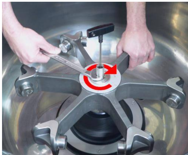
Fig. 21: Fastening of the rotor
