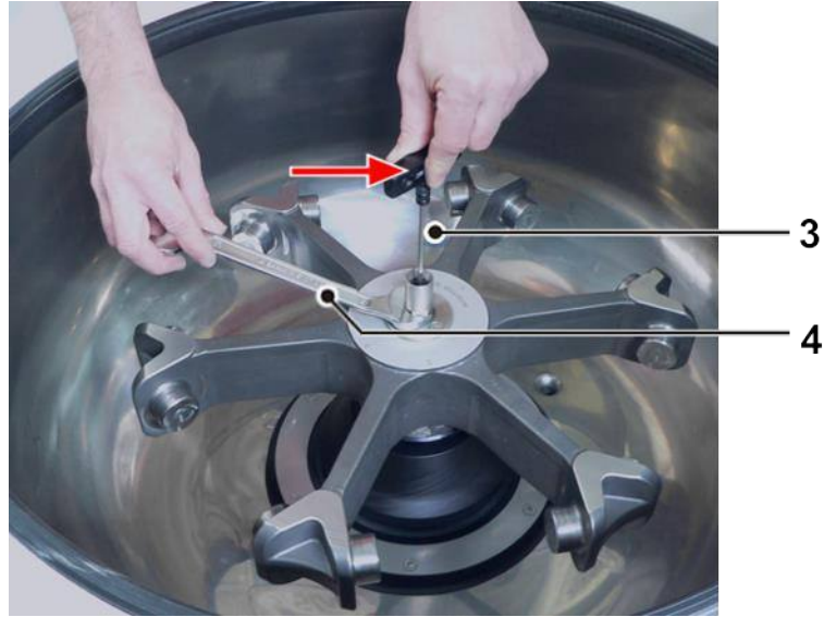
Fig. 20: "Two-finger-principle" for holding the hexagon key
