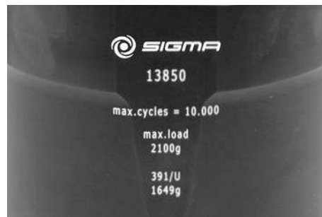
Fig. 8: Different service life – engraving on the bucket/rotor
