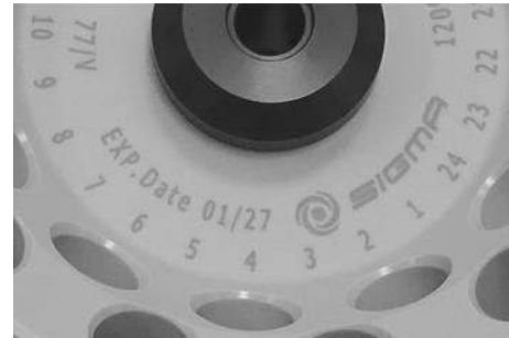
Fig. 8: Different service life – engraving on the bucket/rotor
