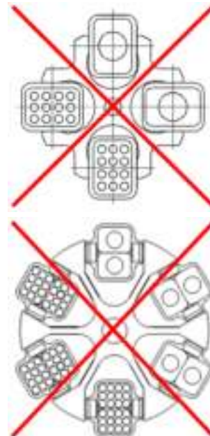
Fig. 8: Permissible and impermissible loading of a swing-out rotor with vessels of various sizes (example illustration)
