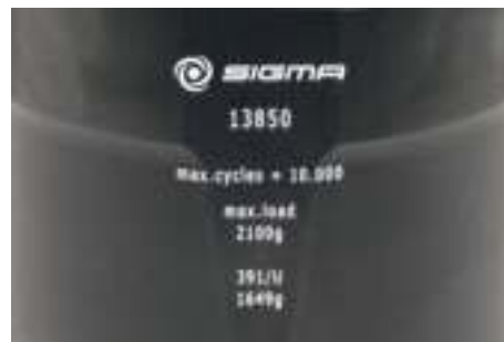
Fig. 4: Different service life – engraving on the bucket/rotor
