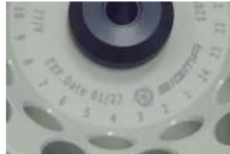
Fig. 4: Different service life – engraving on the bucket/rotor
